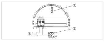
Electronics and terminal compartment, single chamber housing
