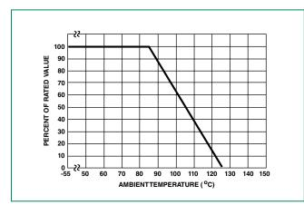
For applications exceeding 85° C, ambient temperatures, the peak surge current and energy rating must be reduces as shown in Figure 1.
