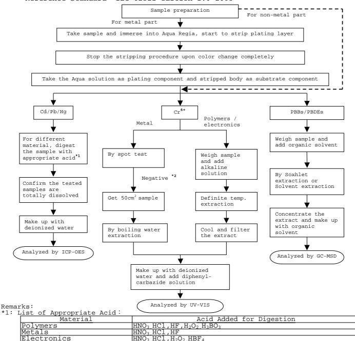
\*2: If the result of spot test is positive, Chromium VI would be determined as detected.
