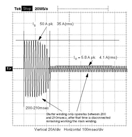
This plot shows the total current flowing through the compressor when it starts to operate and the time in which the current reaches the maximum value (Is) due to the start of the motor. After this time (210 msecs) the start winding
