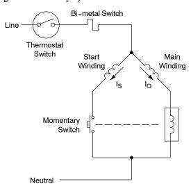
In the previous figure the thermostat-switch is controlling the working-cycle of the compressor and it is dependent on the set point of environment temperature which has to be selected according to the temperature needed. The bi-metal switch protects the compressor against overload and the relay controls the momentary switch which cuts out the starter winding once the motor has reached about 75 percent of the synchronous speed (after around 300 msecs).
