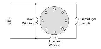
When the line voltage is applied, the current flows through both windings and the result is a rotating stator field which causes the motor to start. At about 75 percent of synchronous speed, the auxiliary winding is cut out by a centrifugal switch.
