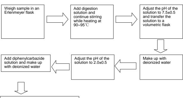
Analyze the mixture by using UV-VIS Spectrophotometer with wavelength set at 540 nm
