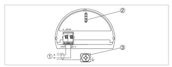
Electronics and terminal compartment, single chamber housing
