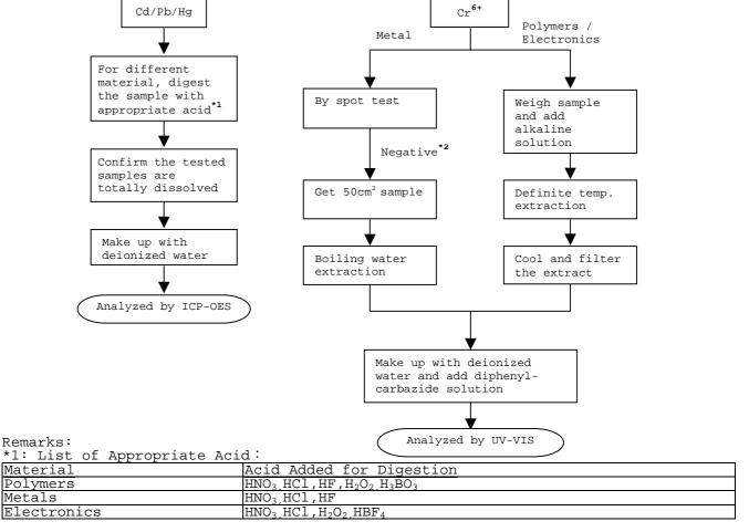
\*2: If the result of spot test is positive, Chromium VI would be determined as detected.
