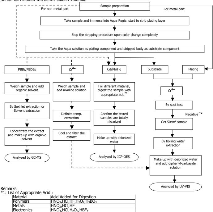
\*2: If the result of spot test is positive, Chromium VI would be determined as detected.
